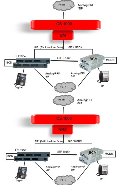
This configuration allows migrating a network of BCM and CS1000 to the IP Office step by step by adding IP Office systems to it.
