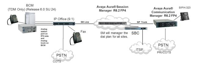
IP Office R9.1 introduces a new deployment scenario for IP Office, where IP Office acts as a SIP Gateway for a Nortel BCM and/or a Norstar telephony system. The following use cases are supported:
