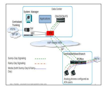
In addition to supporting additional CM features associated within an analog end-point, the ATA will also be able to support an analog Fax end-point.
