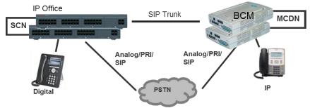
The SIP interoperability support between IP Office and BCM50/450 allows customers to migrate a network of BCM step by step to an IP Office SCN or Server Edition network.
