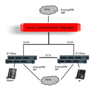
The H323 protocol is used for trunks between the IP Office nodes and the CM. The IP Offices are a network of SCNs and can use advanced SCN feature set between each other.
